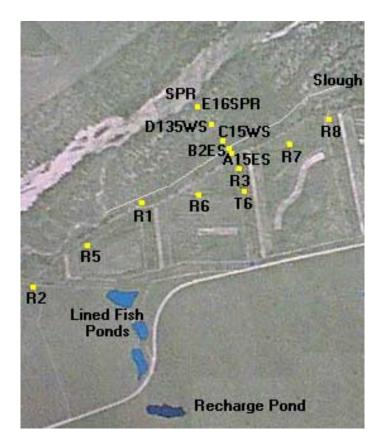
Figure 1. Location of existing pumping wells, slough channels, and South Platte River (SPR). R1, R2, R3, R5, R6, R7, and R8 are pumping wells.
