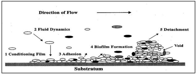
Figure 1-1 Biofilm Formation Diagram (from Precival et al., 2000)]
