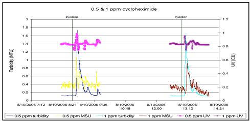
Figure 3-8 Turbidity and UV254 Absorption Response from Biofilm Exposure to Cycloheximide
