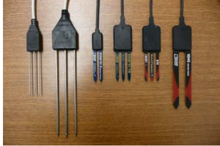
Figure 1. Sensors tested: from left, TDR CS640, CS630, ECH 2 O EC-5, TM, 5TE, and 10HS.
