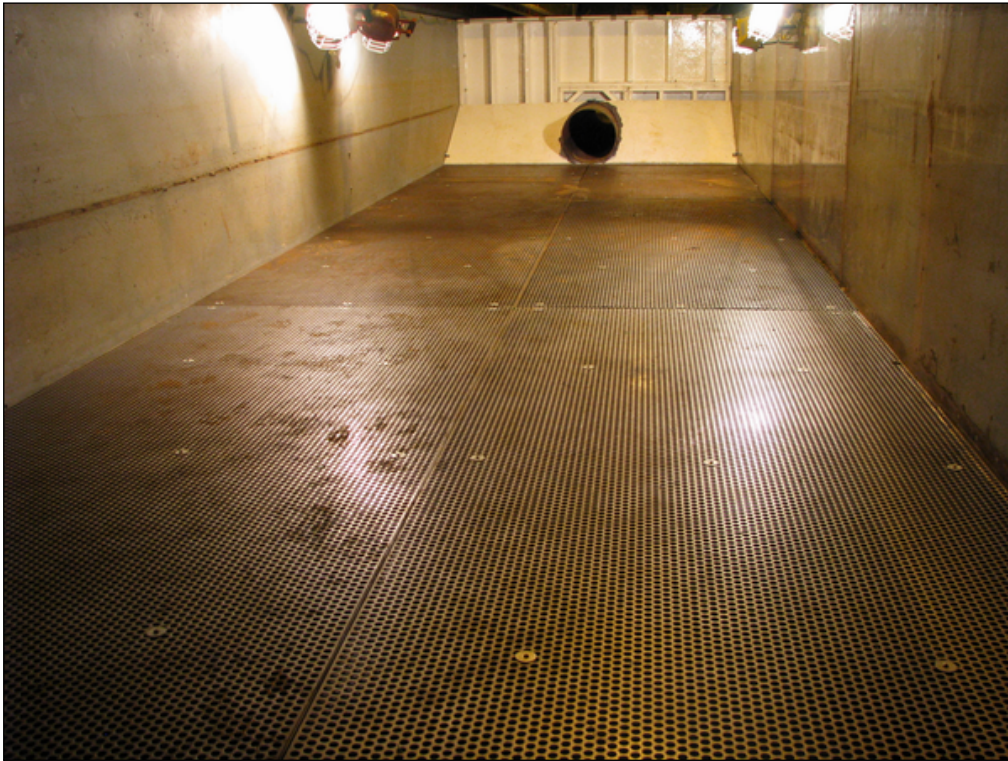
Figure 3. Photograph of 1:4 physical model with simulated unvegetated TM with HPTRM
