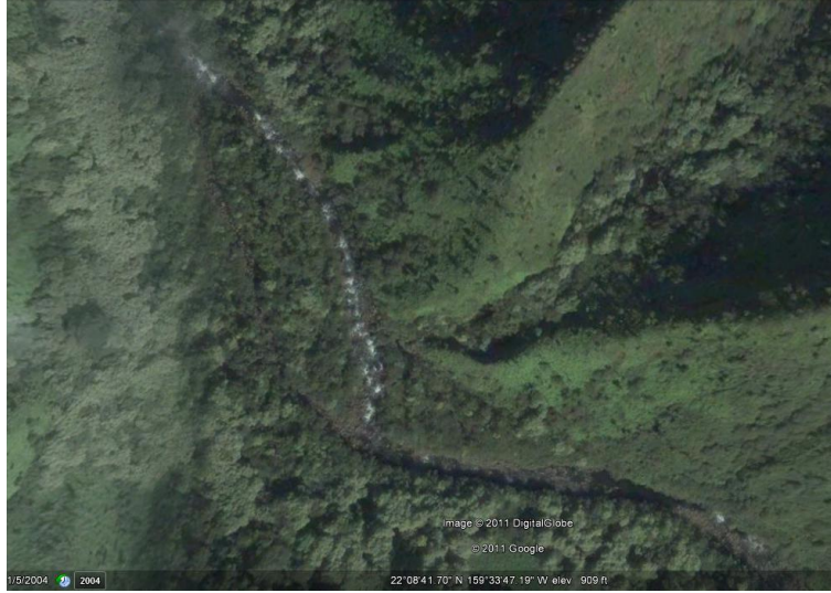
Figure 2. This Google Earth aerial photo is of a section of the Wainiha River of Kauai, Hawaii, just northwest of gaging station 16108000 (see Table 1). This photo shows a bedrock step-pool section of river (left) and a calm section (right). Bedrock step-pool rivers were not identified by Google Earth satellite images and aerial photos alone, but only in conjunction with location photos and personal communication from USGS state hydrologists.
