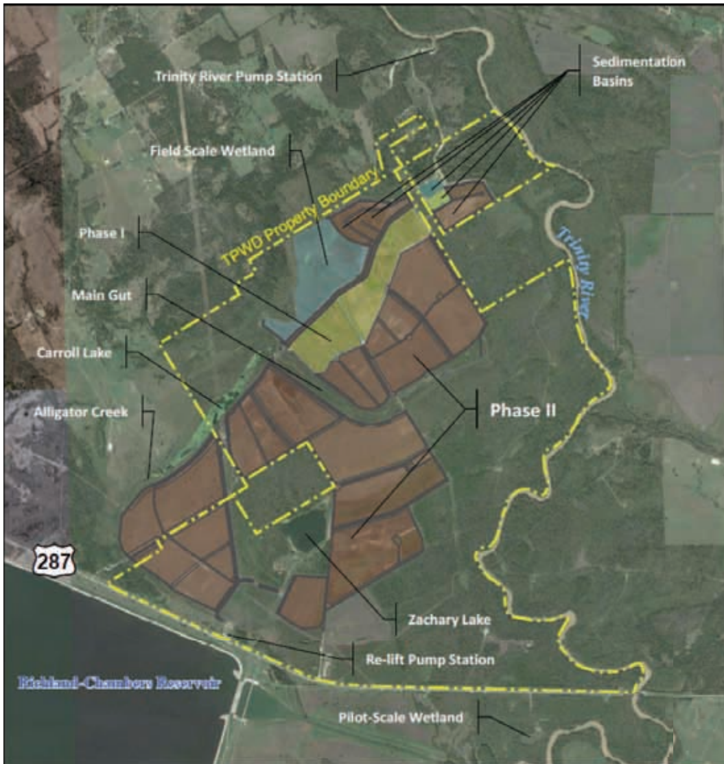
Figure 9. Richland Chambers Wetlands Facility final configuration. (Tarrant Regional Water District, Alan Plummer and Associates, and CH2MHill – Wetlands Commissioning Document)
