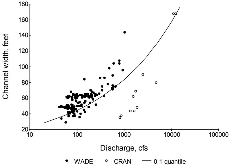
**Figure 7.** Channel width as related to discharge near the gaging station on the Virgin River near Hurricane, Utah for 1993 – 2008. CRAN is measurement made using a bridge crane. The CRAN data was not used to fit the 0.1 quantile relation.
