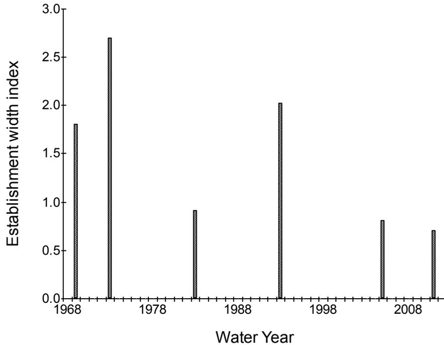
**Figure 8.** Width establishment index for riparian vegetation along the Virgin River near Hurricane, Utah, in the Poudre River, Colorado. The minimum discharge for establishment is 1010 cfs and the power term in the width equation is 0.27.
