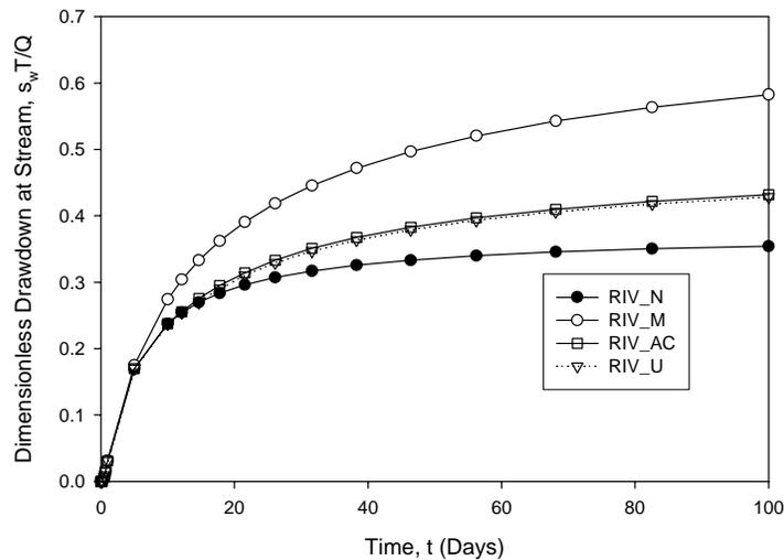
**Figure 5.** Comparison of dimensionless aquifer drawdown at the stream location nearest the pumping well as predicted by the four different MODFLOW RIVER packages for a fine sand aquifer ( $K=5.0 \text{ m-d}^{-1}$ ,  $h_c=50 \text{ cm}$ ).
