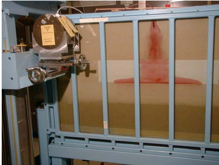
Figure 2. Final carbon tetrachloride distribution in fine-grained sand layer.
