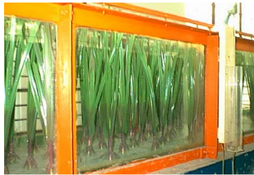
Figure 3. Experimental facilities for vegetated-bed test.
