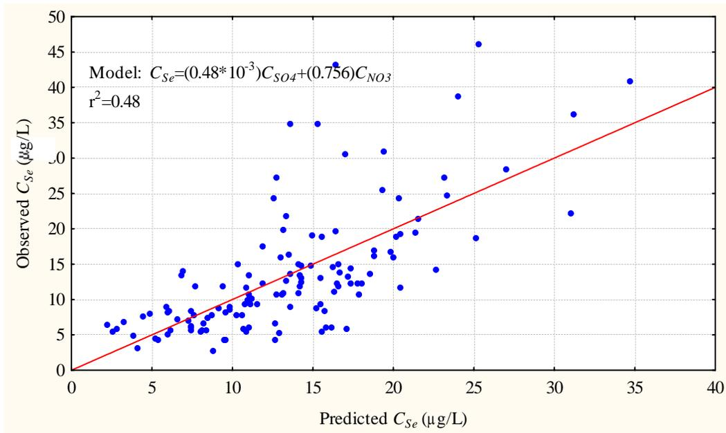
**Figure 12.** Observed Se concentrations in surface water compared to concentrations predicted by a multivariate relationship with SO<sub>4</sub> and NO<sub>3</sub> concentrations.
