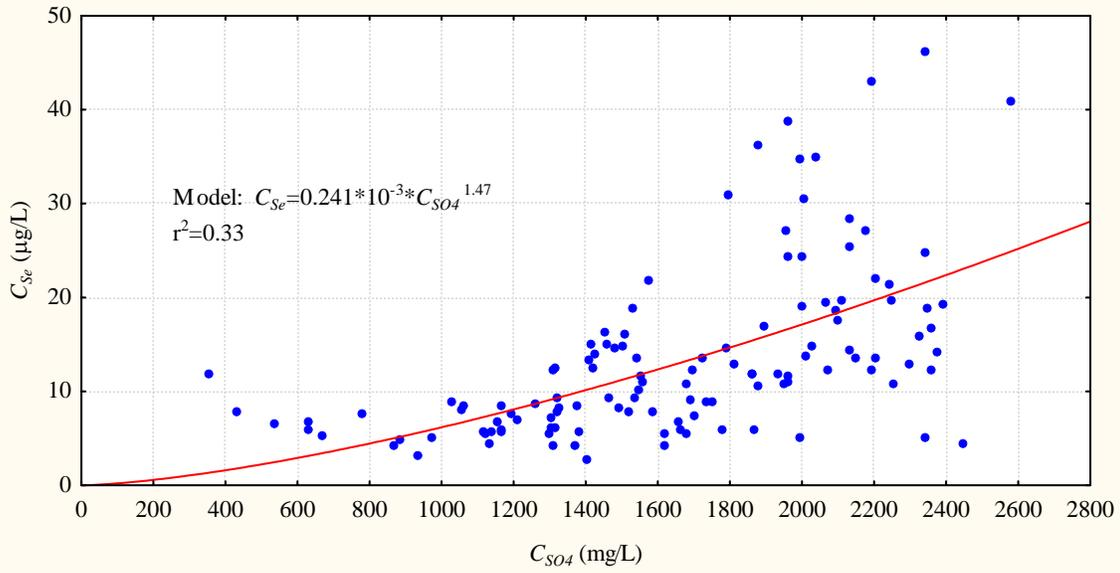
**Figure 11.** Se concentration versus SO<sub>4</sub> concentration for all surface water samples.
