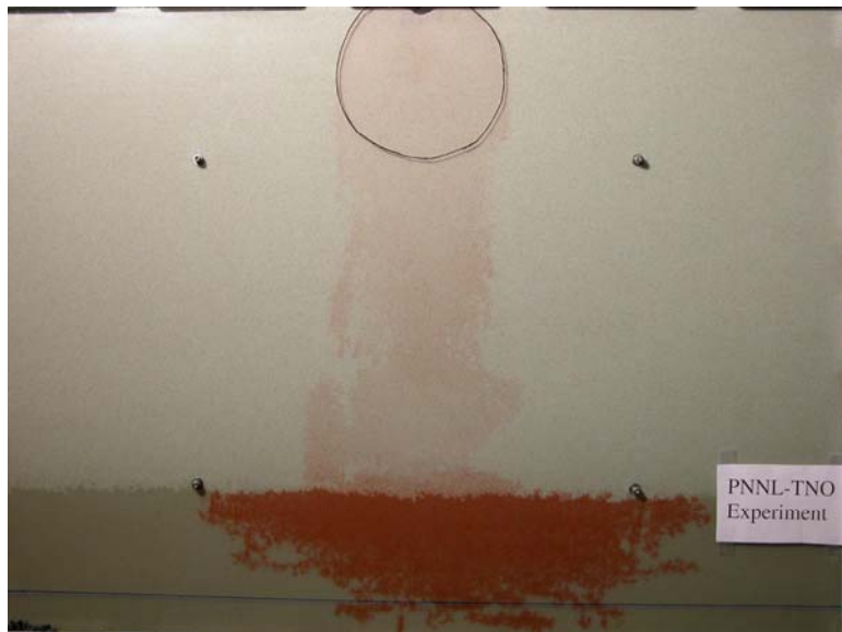
Fig. 2. LNAPL distribution after 30 days.
