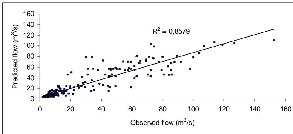
Figure 6. Scatter plot of the observed versus predicted flow with the FFBP networks.
