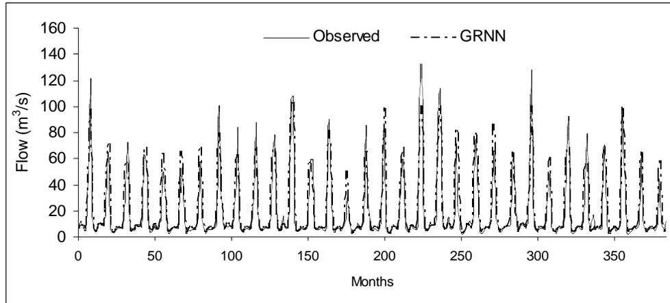
Figure 5. Observed and predicted monthly flow with the GRNN networks.
