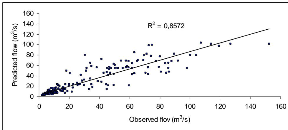
Figure 7. Scatter plot of the observed versus predicted flow with the GRNN networks.
