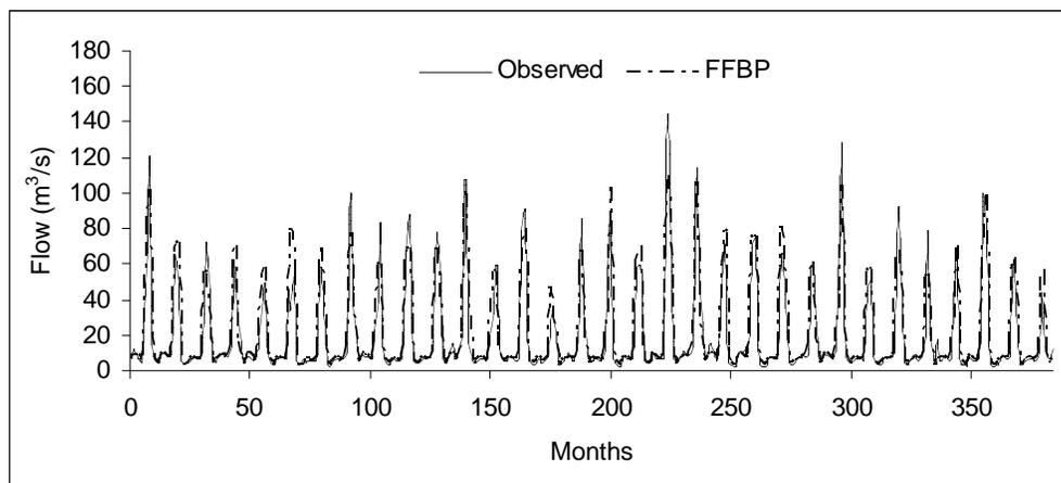
Figure 4. Observed and predicted monthly flow with the FFBP networks.
