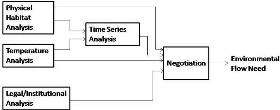
Figure 1. The major components of a typical analysis supporting the application of the Instream Flow Incremental Method (IFIM) to the selection of an environmental flow requirement for management of a water resources system.
