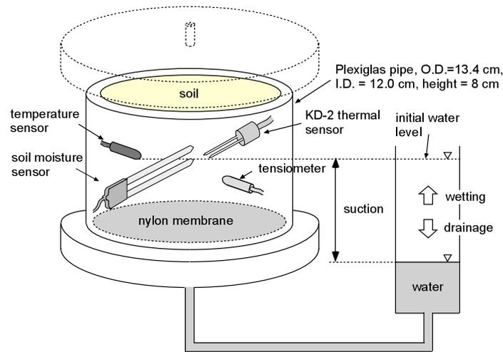
**Figure 1:** Schematic view of the Tempe cell used in the experiments, shown without insulation. The diagram is not drawn to scale. The dimensions of the acrylic pipe are; 8 (height)  $\times$  13.3 (O.D.) cm, wall thickness = 1.27 cm, inside volume excluding the sensors = 909.3  $\text{cm}^3$ .
